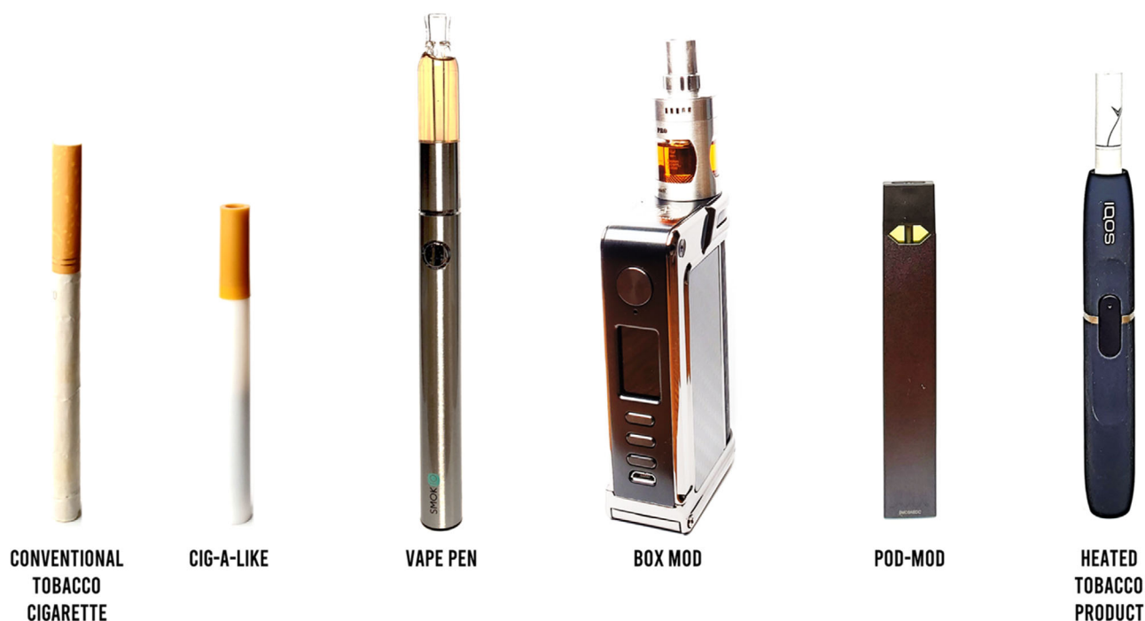
Figure 1. Typical electronic nicotine delivery system (ENDS) devices showing different generations of electronic cigarettes and IQOS, a heated tobacco product.
